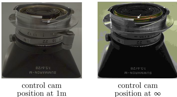
Figure 12: Notch and a control cam on a lens
