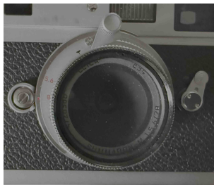
incorrectly mounted lens (lever on the right)
